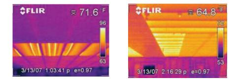
It is seen that ordinary paper is nearly useless in retarding back losses whereas the reflective barrier is effective in reflecting much of the heat that would otherwise be lost. In the thermograph (above right), the material covering the floor joist on the left is aluminum foil backed paper. Its temperature is 64 degrees F. The shorter length of material on the right is ordinary paper without a foil facing. Its temperature is 68 degrees F. This is a considerable difference.
